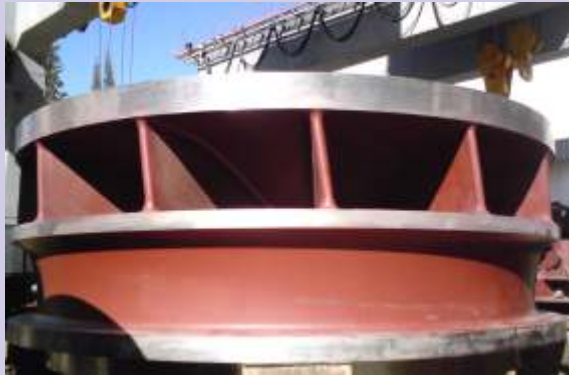
Nurekskaya HPP (Tajikistan): Hydro Turbine under Plant Unit No 3 with Output after Modernization of 345 MW - Modernized Runner at Erection Site (2009)
