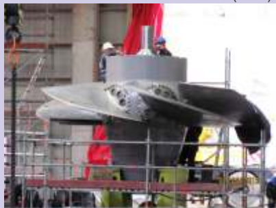
Rucatayo HPP (Chile): 52.9 MW Hydro Turbine – Hydro Turbine Runner at Mounting Site. (2012)
