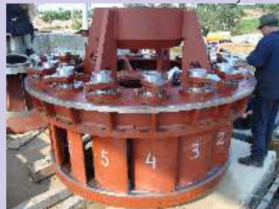
Chicapa HPP (Angola): 4.25 MW Hydro Turbine – Wicket Gate Assembling. (2007)
