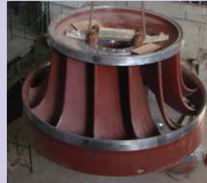
Corumba-3 HPP (Brazil): Hydro Turbine with Output of 47.8 MW – Hydro Turbine Runner at Mounting Site. (2010)
