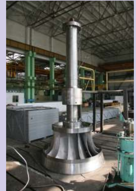
Chicapa HPP (Angola): 4.25 MW Hydro Turbine – Coupling of Hydro Turbine Runner & Shaft at Workshop. (2006)
